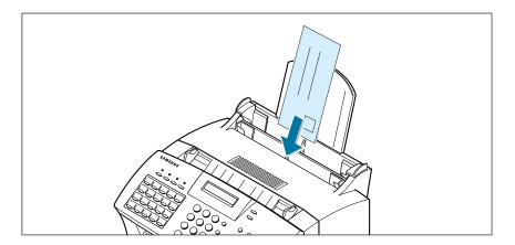
• Load transparencies face up with the adhesive strip on top going into the tray first.
